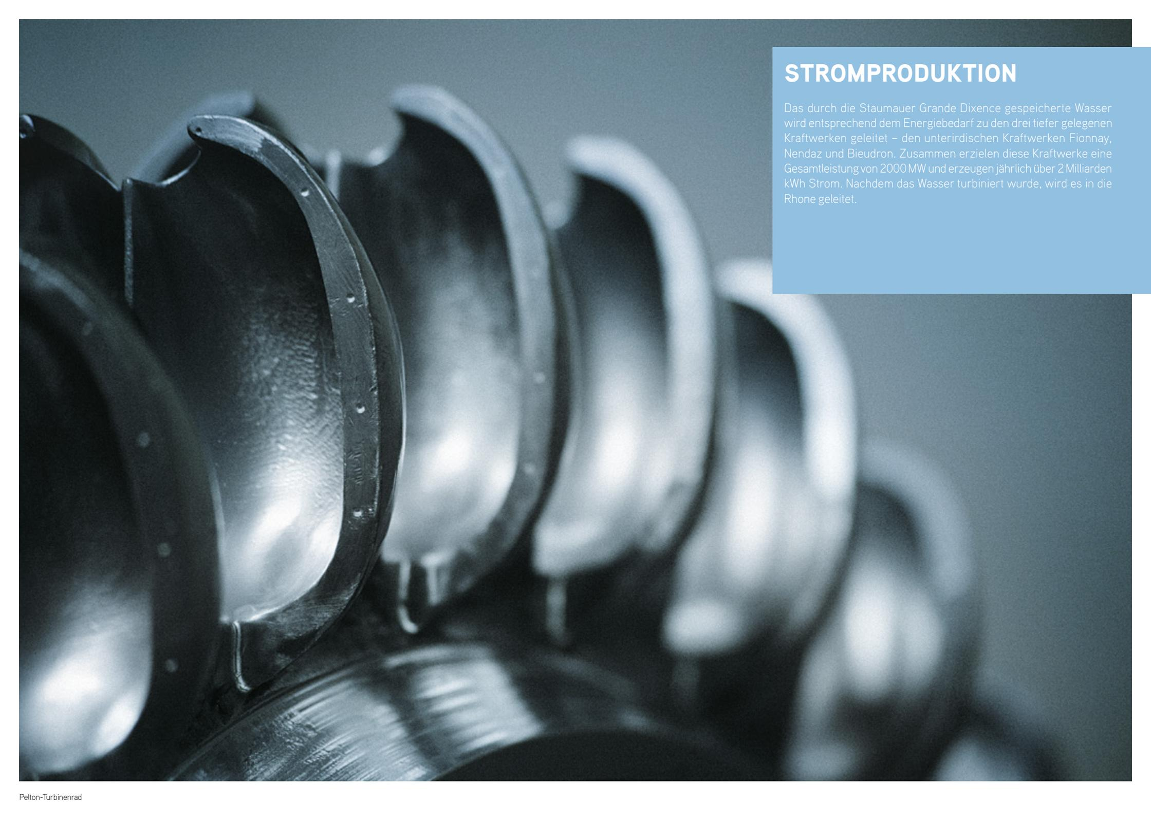
A close-up, black and white photograph of a Pelton turbine wheel. The wheel is composed of several curved buckets arranged in a circular pattern. The buckets are highly reflective, showing bright highlights and deep shadows. The background is dark and out of focus, emphasizing the metallic texture and curved shape of the buckets.
