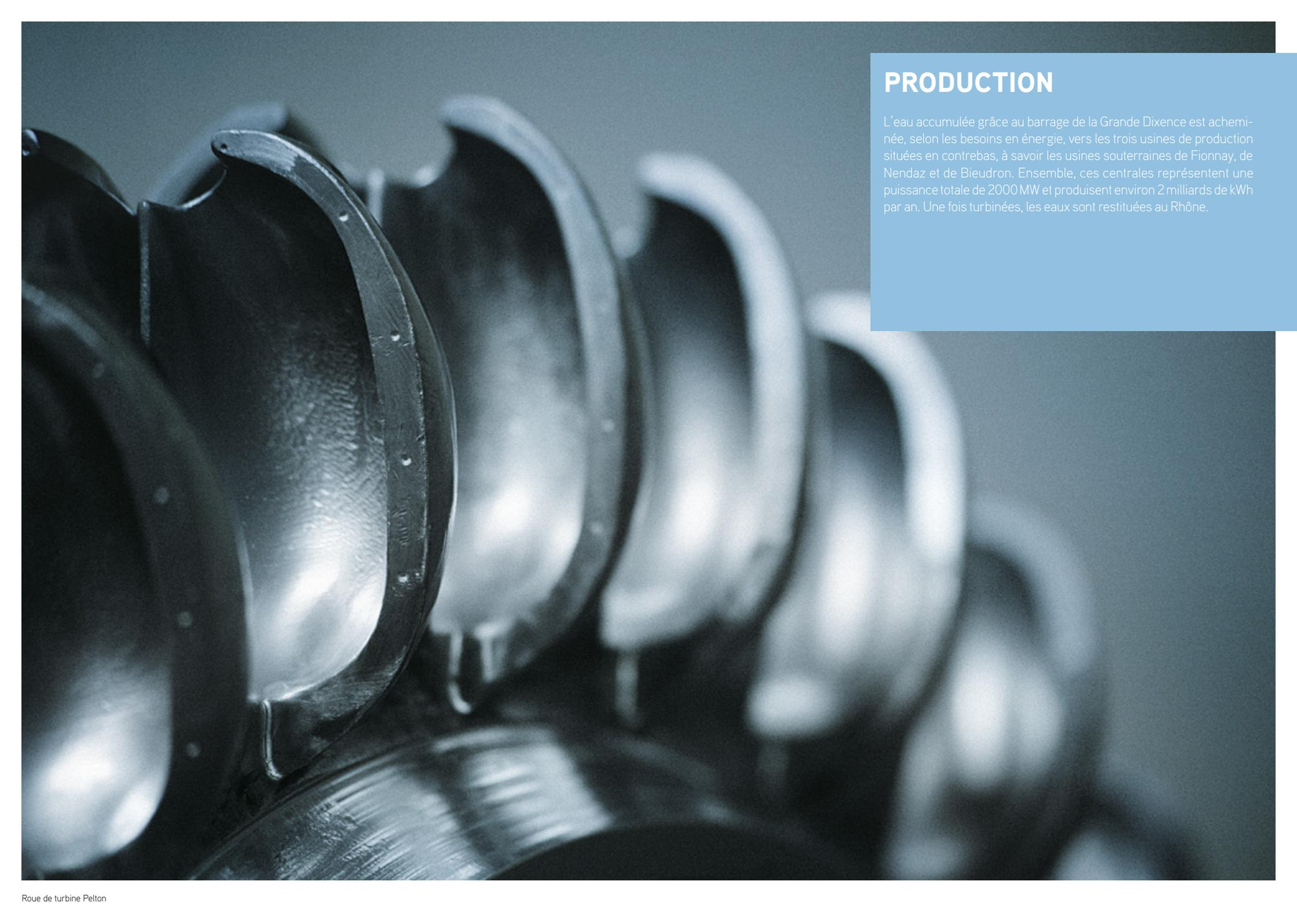
A close-up, black and white photograph of a Pelton turbine wheel. The wheel is composed of several buckets, which are curved and pointed at the bottom. The buckets are arranged in a row, and the lighting highlights their metallic texture and the sharp edges. The background is dark and out of focus.
